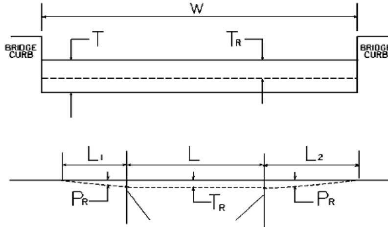
W = bridge width curb to curb                      T = thickness of existing bituminous overlay                      L = length of bridge
