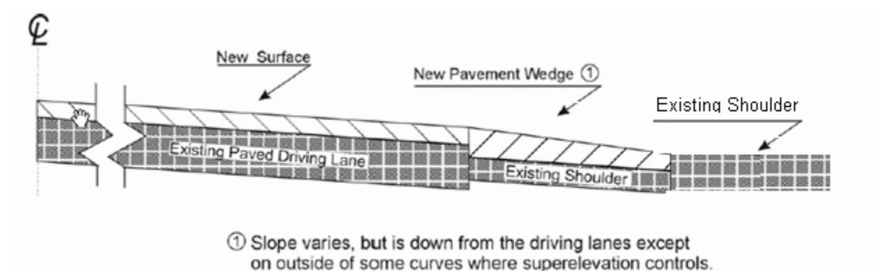
**3.0 MEASUREMENT.** The Department will measure Asphalt Surface Mixture placed as the pavement wedge according to Section 403.
